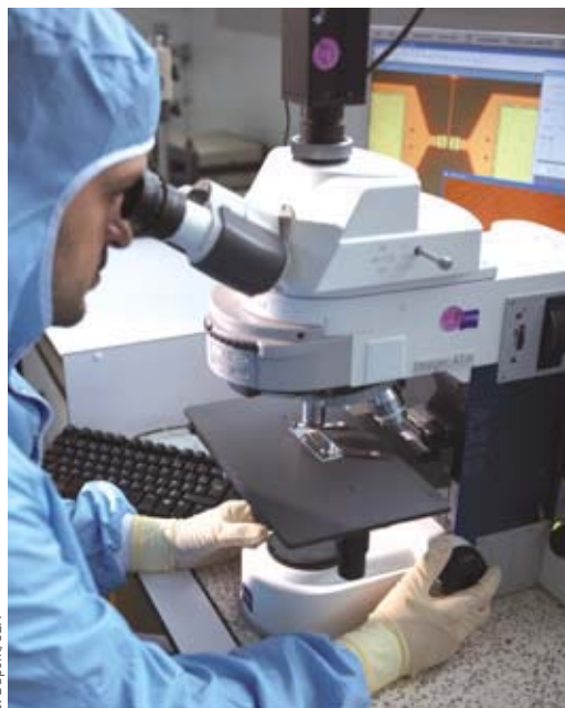
Optical microscope examination of lithographed samples in a clean room Iramis/Spec, CEA Saclay.
